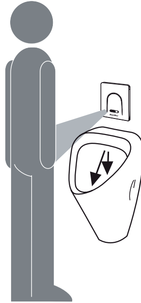
Pre-flushing as required 1 sec. if last flushing took place more than 5 min. ago
