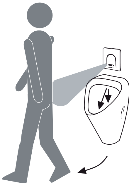
adjustable main flushing cycle from 1 to 10 secs.
